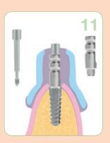
Closed impression method with Standard or individual tray – impression posts for closed impression (Mini, Standard and Large) with the prosthetic screw and transfer cap.
