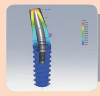
The stability of the implants under load was ensured with FEM analyses and biomechanical tests.
