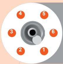
The hexagonal connection allows a high degree of flexibility in orienting the abutment and, therefore, offers the greatest possible freedom for the production of prosthetics. There are 6 possible variations of the abutment-implant position.
