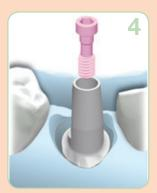
Mark the gingival margin on the model on the abutment, release laboratory screw and remove the abutment. Then remove the excess with a suitable milling cutter. We recommend using a separate laboratory analogue for improved processing (3).
